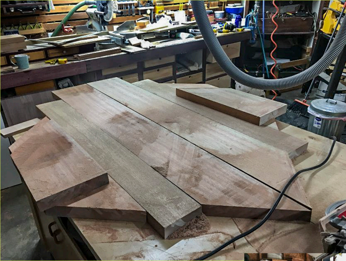
Planks of wood have been glued together to form the base of the chalice.
